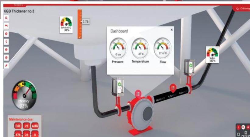
Figure 1 (top). IIoT-equipped flotation loop depicting a smart valve failure. All service history of the valve, manuals, safety documents, drawings and spare parts can be viewed from any smartphone, tablet or PC. Figure 2 (bottom). This IIoT-equipped pumping loop incorporates operation performance measures, future maintenance requirements and overall process measures. (Graphics courtesy of Flowrox)
