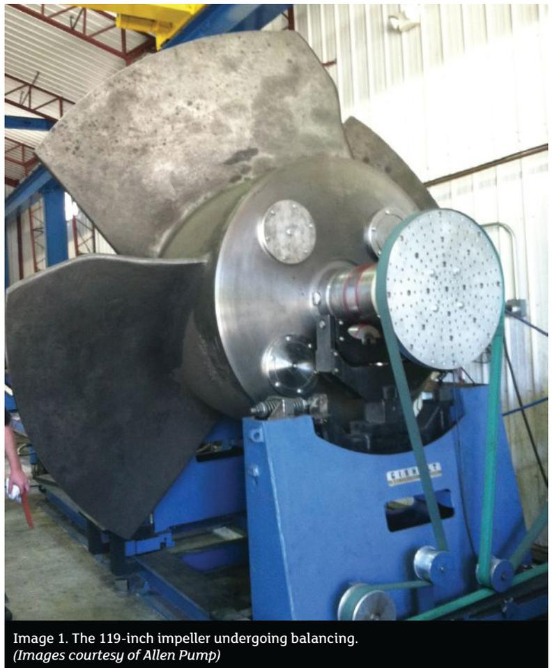
Image 1. The 119-inch impeller undergoing balancing.
