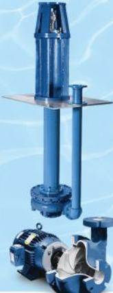
Our vertical sump pump line offers up to 3000 GPM, 230' Heads and 26' depth. The horizontal end suction pump line offers up to 3000 GPM, 300' Heads, back pullout construction and semi-open impellers. Standard construction is Cast Iron, 316 Stainless Steel fitted, or all 316 Stainless Steel, and the self-priming pump is available in CD4MCu.
