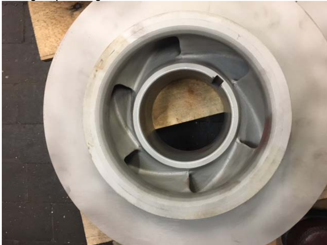
1 st Stage Impeller in good condition
