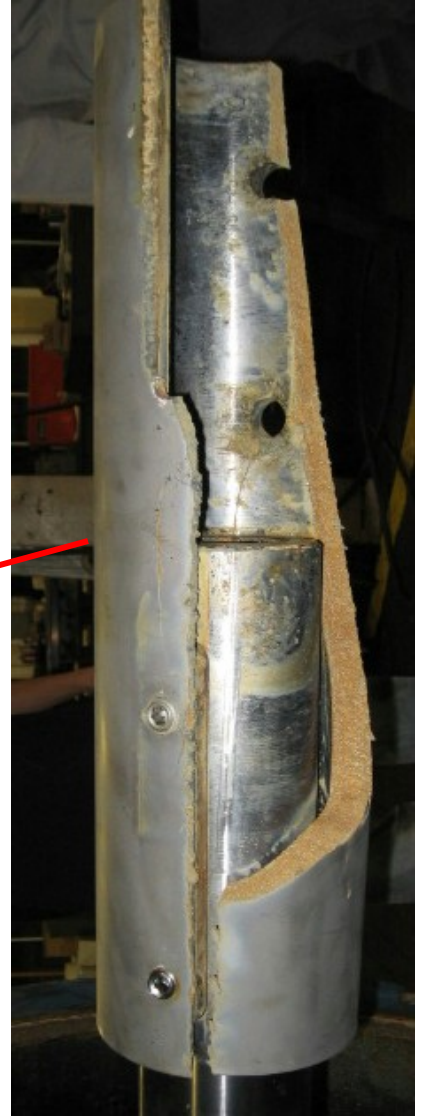
Internal Shaft coupling fracture at keyway
